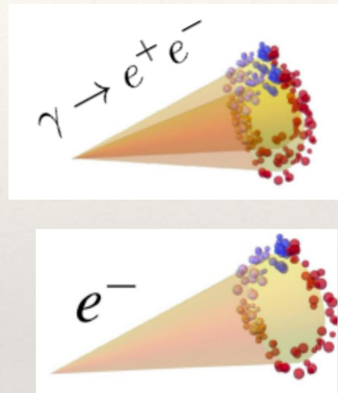
Cannot distinguish between Cherenkov cone of electrons and single photon
